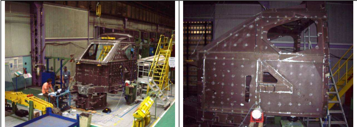
Figure 9: Experimental modal analysis setup of the driver's cab BIW
