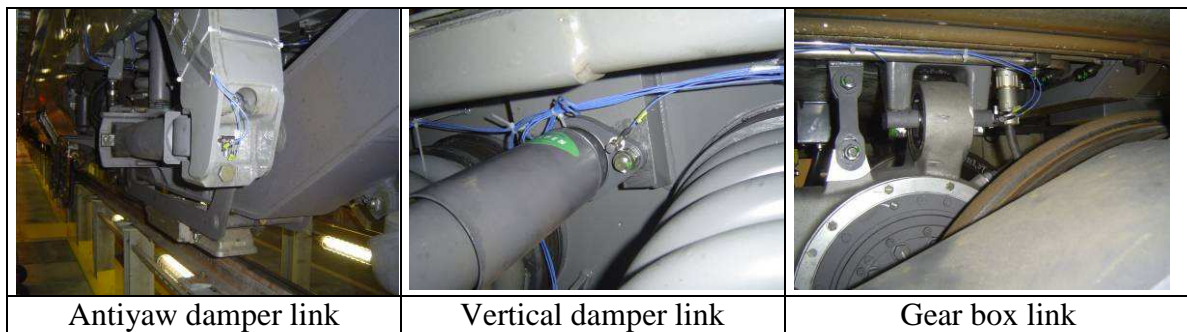
Figure 2: Example of structureborne paths measured
